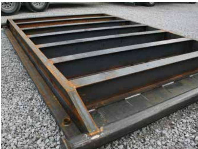
Image 3. A key to effective VRU operation in the oilfield is the skid on which it rests. This skid assembly must be the proper weight and anchored correctly if it is to effectively absorb the shaking forces that are produced by the VRU's compressor.
