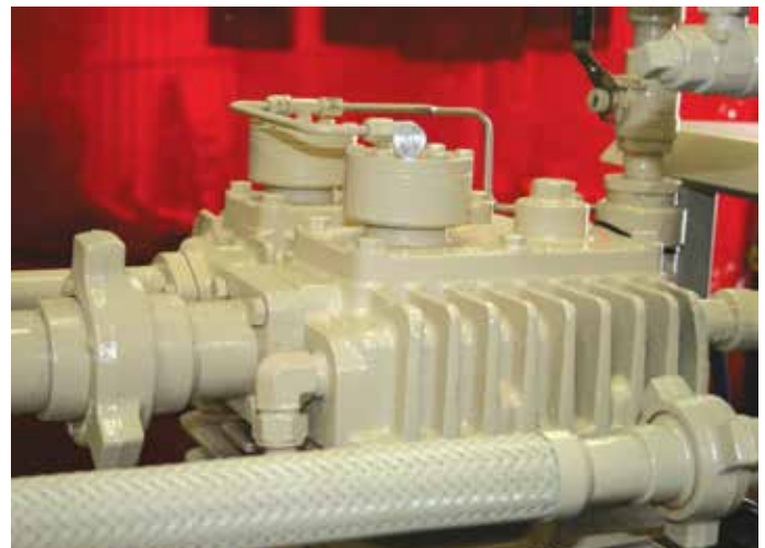
Image 4. All reciprocating-type compressors produce shaking forces. If the compressor is not installed correctly, those shaking forces will create vibrations that can harm the performance of the compressor and VRU.
